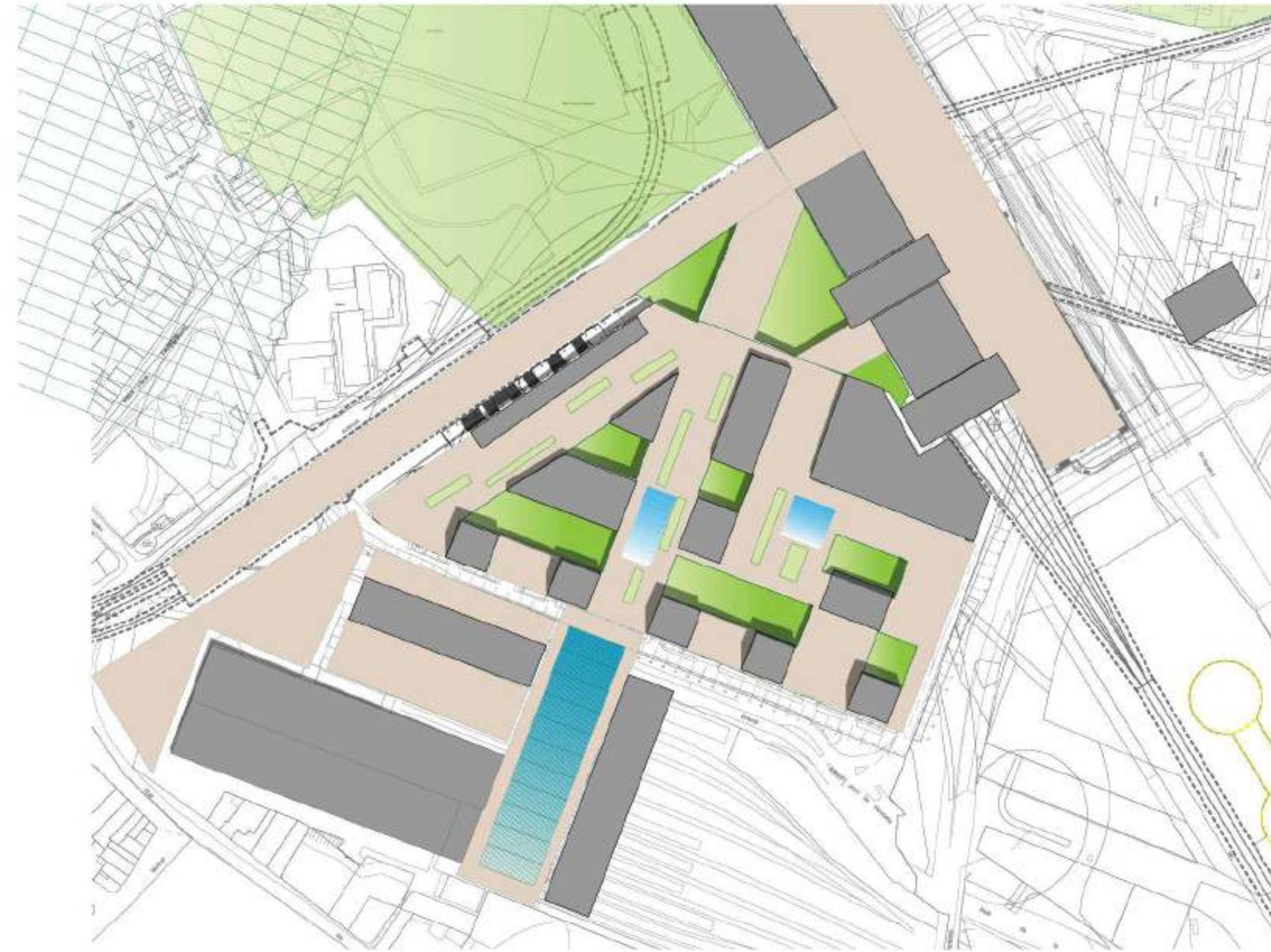
ROOF PLAN Densification in height to compensate the loss of built area due to the reshaping of the basement.
